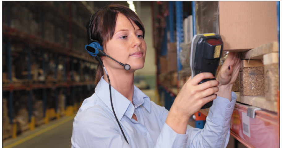
Hand-held EDI 3G bar code reader – typical of the many devices that require shielding.
