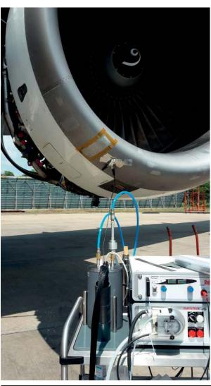
ention "brush plating" and it conjures up images of a primitive process using plating solution taken from a tank and applied using a powerpack attached to a swab. This is an outdated notion of the process. With modern techniques, selective electroplating on a small scale can be a key weapon in the surface treatment armoury.
