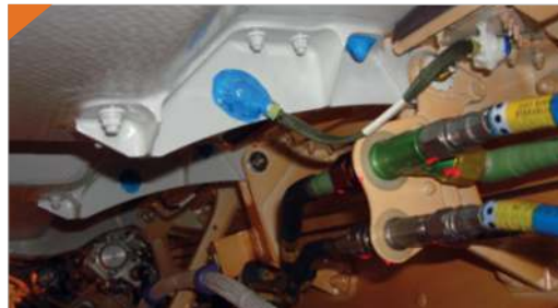
FIG 1: ELECTRICAL BONDING POINT ENCAPSULATED IN NYCOTE 7-11 BLUE
